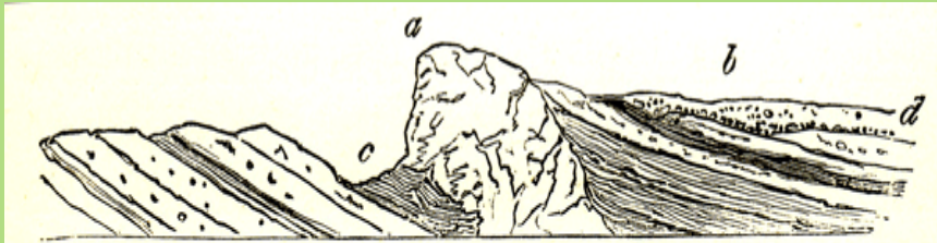
FIG. 82.—Section of the form of hill in the Lowlands of Scotland known as 'Crag and Tail.' a , 'Crag' of basalt or other eruptive rock. b , 'Tail' of softer rocks which have been worn away from around the hard igneous mass. c , Hollow often found in front of the crag. d , Covering of drift.
