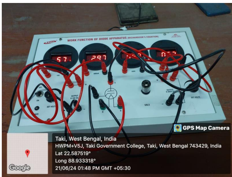
Apparatus for Determination of a Work Function of the Filament Metal of a Vacuum Diode
